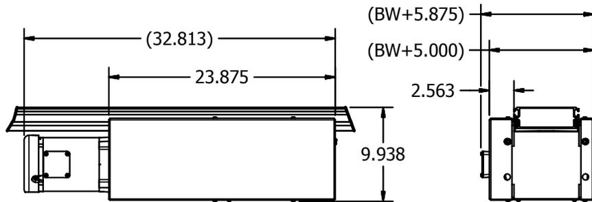
**DRIVE #20** Center Drive • Frame Mount • Right Angle • Infeed Facing
