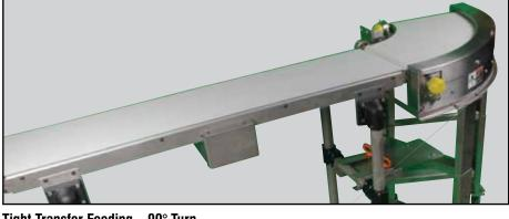
Multiple belts with one drive for special parts handling.
